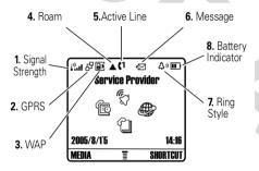
1 **Signal Strength Indicator** – Vertical bars show the strength of the network connection.
