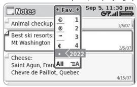
Use the D-pad or trackball to navigate through the list: left-right to flip through the Favorites, Recent, alphabet, and symbol sets; up-down to select specific characters. Press the trackball to insert a highlighted character. Here are some useful tips in using the Special Character selector:
