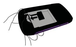
4 To remove the SIM card, pull the card straight out along the long, exposed edge. You may need to use a tweezers to grip the card. Once enough of the card is free of the bracket, gently slide the card out and remove.
