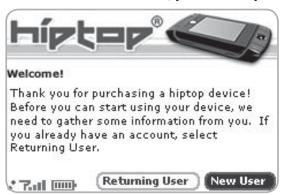
Press the trackball to select the **New User** button and advance to the next screen. On subsequent screens, select the **Next** button to advance.
