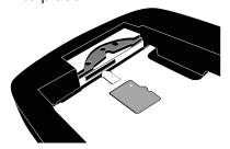
4 To eject the memory card, push the card in slightly and release; the card should spring partly out of the slot. Pull the card free of the device.
