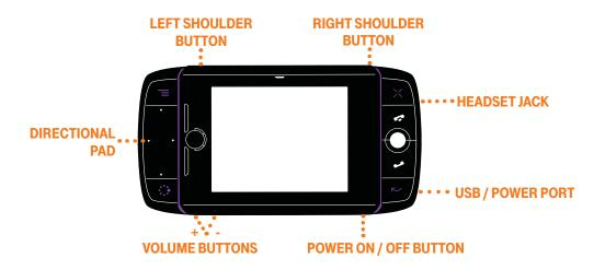
**DIRECTIONAL PAD (D-Pad)** Press up, down, left, or right to scroll or move within text fields, and navigate in games. The D-Pad "rocks" in four different directions and generally mirrors the behavior of the trackball.
