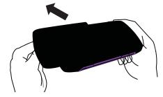
3 Lift the battery from the edge closest to you and remove. You may need to use your nails to grip the battery.
