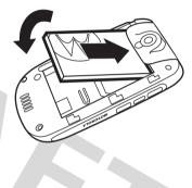
Slide the battery down toward the bottom of the battery compartment to lock it in place.
