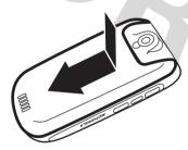
Insert the battery under the tab at the top of the battery compartment. Push the battery up under the tab and lower it into the battery compartment.
