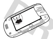
Place the battery door on the phone and slide it up to lock shut.
