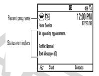
Press  $\mathbf{\hat{\phi}}$  right/left to scroll through the application shortcuts, and press  $\mathbf{\hat{\phi}}$  down/up to scroll through the status fields. Press  $\mathbf{\hat{\phi}}$  to select an item.
