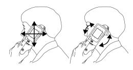
If your HA has a telecoil, activate its switch, then also rotate the handset as illustrated to align the telecoils.
