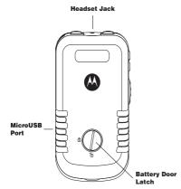
Your phone is water resistant and can be immersed in up to one meter of water for no more than 30 minutes.
