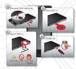
1 Insert the SIM tray removal tool into the hole to unlock the SIM card tray, then slide the SIM card tray out of the phone.
