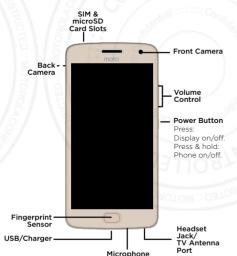
Put in the nano SIM and memory cards. Put the SIM cards into the tray With phone facing included with your Turn tray over to put in an phone into the hole in optional microSD card. the SIM tray to pop out the trav microSD **8** Nano SIM Push tray back into your phone.
