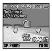
Labels at the bottom corners show the current soft key functions. Press the left soft key ( ) or right soft key ( ) to perform the function indicated by the left or right soft key label.
