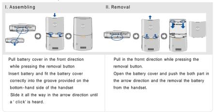
Before removal the battery, be sure to turn off the power of the phone. Forcible removal of the battery may cause malfunction. Cell phone and battery cover shall be always combined.
