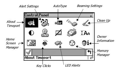
Press the NAVDISC down to see all of the application icons on the Control Panel. To select applications in Control Panel, press the TAB key to highlight the application, then press ENTER to open the application.
