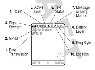
**1. Data Transmission Indicator** Shows connection and data transmission status. Indicators can include:
