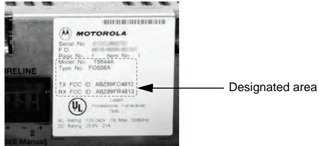
Figure 10-5 Location to affix the Digital Upgrade Kit label
