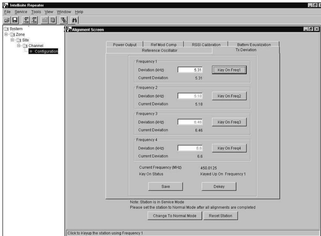
TUNE-UP PROCEDURE - Reference Modulation Compensation Alignment Screen
