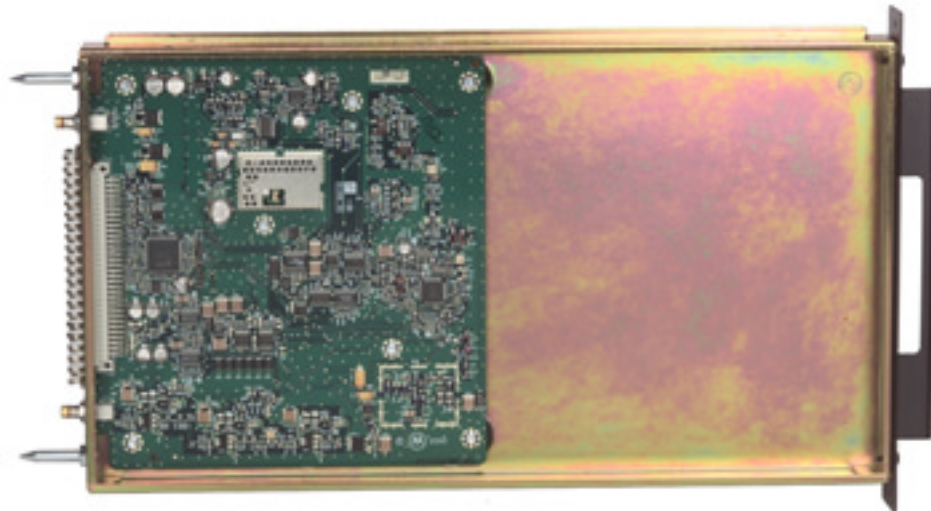
Figure 3 Low Noise 800 MHz Exciter (with cover removed)
