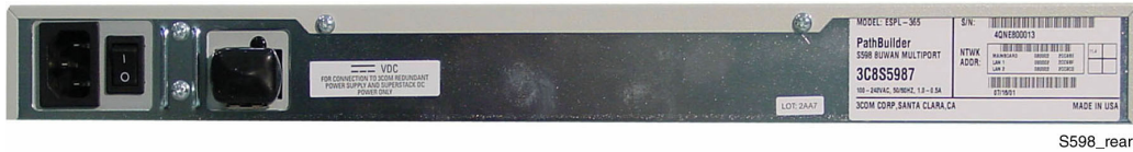
Figure 5-21 Rear View of the Simulcast Remote Site Router
