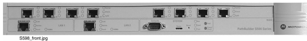
Figure 5-20 Front View of the Simulcast Remote Site Router
