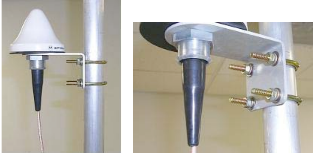
Figure 9: Detail of GPS antenna mounting
