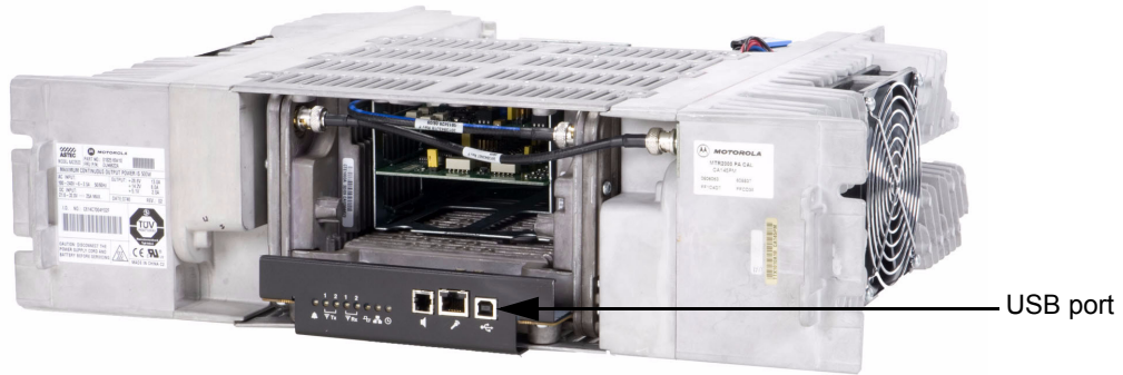
Figure 13-2 Front view (without front bezel) of MTR3000 Base Station/Repeater
