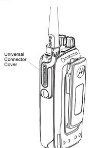
Place the universal connector cover loop over the attached antenna. Slide it all the way down to the base of the antenna.
