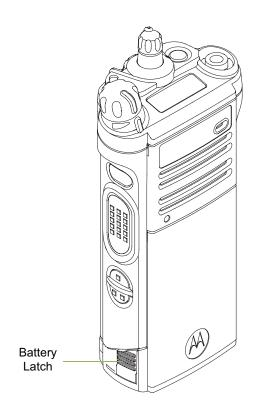
To remove the battery, turn the radio off. Squeeze the release latches on the bottom of the battery until the battery releases from the radio. Remove the battery from the radio.
