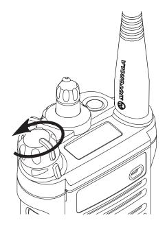
To turn off the radio, rotate the **On/Off/Volume Control Knob** counterclockwise until you hear a click.
