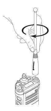
To remove the antenna, turn the antenna counterclockwise. Make sure you turn off the radio first.
