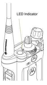
The LED lights up solid red while the radio is transmitting, and solid yellow when the radio is receiving a transmission (conventional mode only). There is no LED indication when the radio receives a transmission in trunking mode.
