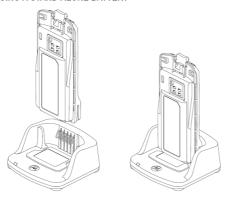
To charge only the battery - at step 4, insert the battery into the tray, with the inside surface of the battery facing the front of the charger, as shown. Ensure the slots in the battery correctly engage in the charger
