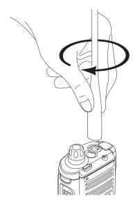
To remove the antenna, turn the antenna counterclockwise. Make sure you turn off the radio first.
