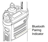
**Note:** Bluetooth range of operation is 10 meters line of sight. This is an **unobstructed** path between the location of
