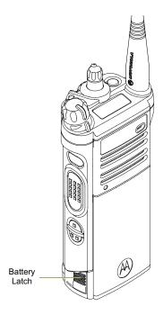
To remove the battery, turn the radio off. Squeeze the release latches on the bottom of the battery until the battery releases from the radio. Remove the battery from the radio.
