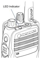
**Solid green** – Radio is transmitting. Also indicates full charge of the battery when the programmed **Battery Strength** button is pressed.
