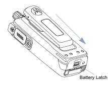
To remove the battery, turn the radio off. Move the battery latch into unlock position and hold, and slide the battery down and off the rails.
