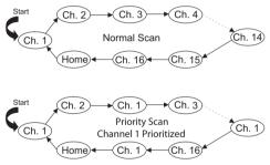
During scan, when activity is detected that meets the unsquelch condition, the radio stops scanning and switches to that channel; the  $\swarrow$  indicator is illuminated, and the channel number is displayed. When no activity is detected for a pre-set time, the radio resumes scanning.
