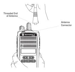
To attach, fasten the antenna to the radio by placing the threaded end of the antenna into the Antenna Connector and rotate clockwise until tight. To remove, turn the antenna in a counterclockwise direction until it disengages from the radio.
