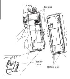
To attach, fit the battery slots with the grooves on the radio and slide the battery upwards until a click is heard. To remove, slide the battery latch away from the radio, slide the battery downwards and pull it away from the radio.
