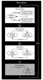
NOTE: For single channel models, only Monitor is available from Menu list. To activate, press and hold the Menu Button; to deactivate, press and hold the Menu Button again.
