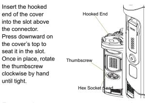
To remove the accessory connector cover, rotate the thumbscrew counterclockwise until it disengages from the radio. If the thumbscrew is too tight, use an Allen wrench to loosen it first.
