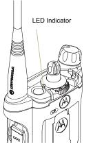
The LED lights up solid red while the radio is transmitting, and solid yellow when the radio is receiving a transmission (conventional mode only). There is no LED indication when the radio receives a transmission in trunking mode.
