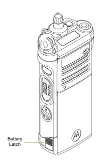
To remove the battery, turn the radio off. Squeeze the release latches on the bottom of the battery until the battery releases from the radio. Remove the battery from the radio.
