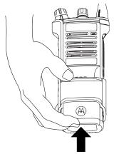
To remove the radio from the carry holder, place the tip of your fingers on the ledge of the carry holder and push at the bottom of the radio until the radio releases from it.
