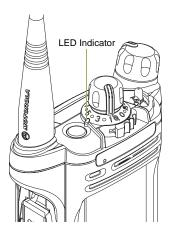
The LED lights up solid red while the radio is transmitting, and solid yellow when the radio is receiving a transmission (conventional mode only). There is no LED indication when the radio receives a transmission in trunking mode.
