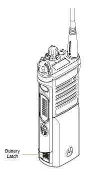
To remove the battery, turn the radio off. Squeeze the release latches on the bottom of the battery until the battery releases from the radio. Remove the battery from the radio.
