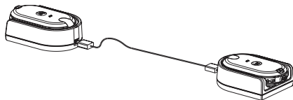
Cloning the Radio through a Single Unit Charger
