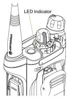
**Blinking yellow** – Radio is receiving a secured transmission.
