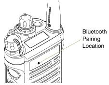
The range of Bluetooth operation is 10 meters line-of-sight communication. This is an **unobstructed** path between the location of the signal transmitter (your radio) and the location of the receiver (your device or accessory).
