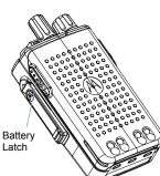
To remove the battery, turn the radio off. Move the battery latch into unlock position and hold.
