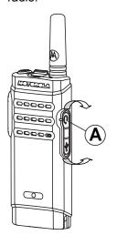
Lift up the flap of the Audio Jack cover. Align the indicators (ⓐ) on both the connector and housing, then push until it fits in properly.
