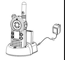
The drop-in charger will also sequentially charge a spare SNN5571 Li Ion battery. The spare battery will not begin to charge until the radio battery is fully charged. Both batteries will charge in approximately 2 to 6 hours.
