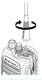
Turn the antenna clockwise to attach it.
