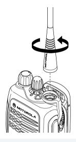
Turn the antenna counterclockwise to remove it.
