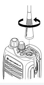
Turn the antenna counterclockwise to remove it.
