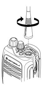
1 Turn the antenna clockwise to attach it.
