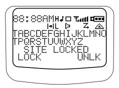
The above screen example may not be identical to the display symbol arrangement in your radio. The top two screen rows display menu and radio status information.
