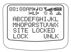
The above screen is typical of what you will see on your radio. The 64 x 96 pixel liquid crystal display (LCD) shows radio status, text, and menu entries. The top two screen rows display radio status, the middle rows show text for messages and other information, and the bottom row contains menu entries.
