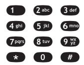
The 3 x 4-key alphanumeric keypad provides an interface to your radio's features. It is arranged similar to a standard telephone keypad.
