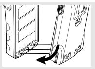
2 Press the top of the battery against the radio until it clicks into place.
