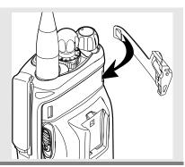
2 Snap the larger end of the adapter into place in the shroud indent, below the antenna port.
