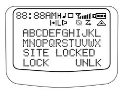
The above screen is typical of what you will see on your radio. The  $64 \times 96$  pixel liquid crystal display (LCD) shows radio status, text, and menu entries. The top two screen rows display radio status, the middle rows show text for messages and other information, and the bottom row contains menu entries.
