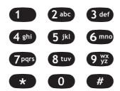
The 3 x 4-key alphanumeric keypad provides an interface to your radio's features. It is arranged similar to a standard telephone keypad.
