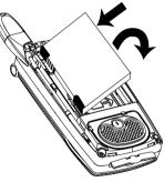
3 To replace the battery door, locate the tabs on the battery door and the slots in the phone.
