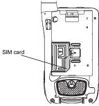
If your SIM card is not in the SIM card holder, it may be in the box your phone came in, attached to a piece of plastic about the size of a credit card. If this is the case, carefully detach your SIM card from the surrounding plastic and insert it as described in "Inserting Your SIM Card" on page 19.
