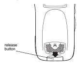
3 Allow the battery door to pop up, slide it forward, and remove it from the back of your phone.
