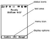
The screen shown is the idle screen. The text that appears on your idle screen depends on your service provider. The idle screen appears when your phone is on, but not engaged in any activity.
