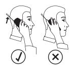
Important: Failure to fully extend or retract the antenna until the antenna clicks into place causes severely degraded performance, which may result in missed calls, dropped calls, or garbled audio.
