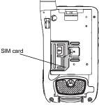
If your SIM card is not in the SIM card holder, it may be in the box your phone came in, attached to a piece of plastic about the size of a credit card. If this is the case, carefully detach your SIM card from the surrounding plastic and insert it as described in "Inserting Your SIM Card" on page 16.
