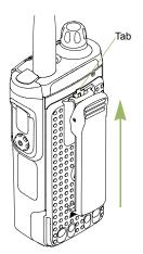
To remove the clip, use a flatbladed object to press the belt clip tab away from the radio. Then, slide the clip downward and away from the radio.
