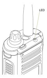
The LED lights up solid red while the radio is transmitting. In conventional mode, the LED lights up solid yellow when the radio is receiving a transmission. In trunking mode, there is no LED indication when the radio receives a transmission.
