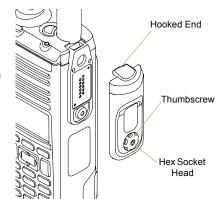
To remove the accessory connector cover, rotate the thumbscrew counterclockwise until it disengages from the radio. If the thumbscrew is too tight, use an Allen wrench to loosen it first.
