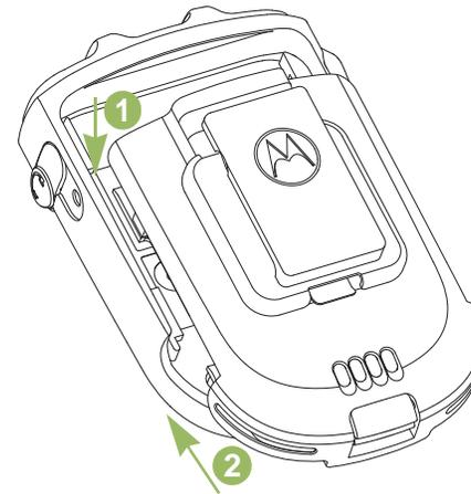
Figure 2.2: Attaching the battery into the WRSM
