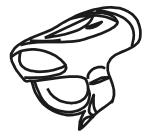
The Emerald ring scanner is designed to be worn on the second and third fingers of the hand that is used to scan the tracking number. The scan window should be facing out. The battery should be slotted on the underside of the ring scanner.
