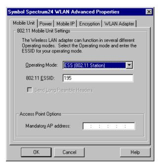
ESS (802.11 Station) - Select ESS (802.11 Station) to enable the MU to transmit and receive data with an access point. The data rate is based on transmit retries. When a data rate is not achieved the MU defaults to the next highest selected data rate. ESS is the MU default mode.
