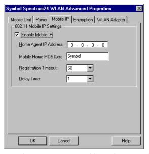
Enter the Home Agent AP Address of an AP on the home subnet. This enables the MU to register with a foreign subnet access point and tell the access point where the MU home access point is located.
