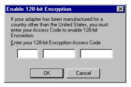
Once 128-bit Encryption is enabled, select 128-bit Encryption from the Encryption Algorithm pull-down menu and enter a 26 Hex digit password for each Encryption key. The password can be entered by spreading the 26 Hex digit password across the six fields provided for each Encryption key. Click OK to save and implement the password for the Encryption keys.
