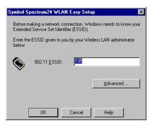
Clicking the Advanced button allows users to view or edit WLAN adapter settings using the Mobile Unit, Power, Mobile IP, Encryption and WLAN Adapter property pages.
