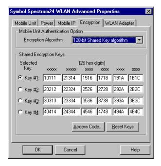
Use the Encryption Algorithm pull-down menu to select the Open System, 40-bit or 128-bit Encryption algorithm to be used for the adapter. The Open System algorithm (default setting) does not encrypt packets over the network. Select Open Systems to disable Encryption for the WLAN adapter and allow for the transmission and receipt of data with no security.
