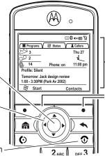
**5.** Press the left /right soft keys to open the screen menus. The menu label of the soft key is displayed at the bottom of the screen.
