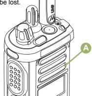
Your radio is designed to be submerged to a maximum depth of 6 feet, with a maximum submersion time of 2 hours.
