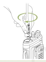
**3** To remove the antenna, turn the antenna counterclockwise.
