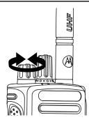
Increase the volume by turning the **On/Off/Volume Control Knob** clockwise.
