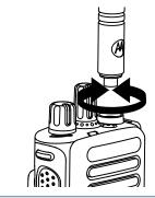
**2** To remove the antenna, turn the antenna counterclockwise.
