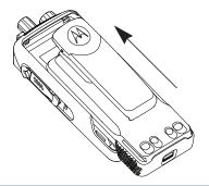
**2** To remove the battery, turn the radio off. Move the battery latch (ⓐ) into unlock position and hold, and slide the battery down and off the rails.
